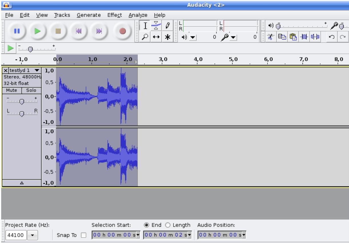
Now the volume on this recorded segment is corrected. This is a better way to be sure that the record you have done not are overdriven, so have to Low setting and afterwards let audacity fix the volume on it.
